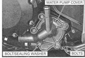
Remove the water pump cover assembly Remove the O-ring from the water pump body.
