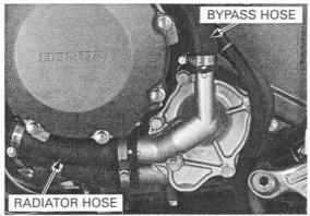
Remove the flange bolts, sealing washer.
