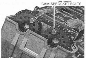
Remove the bolts and CMP sensor rotor from the exhaust camshaft.
