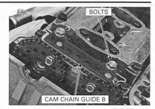
It is not necessary to remove the cam sprocket from the camshaft except when replacing the camshaft and/or cam sprocket.
