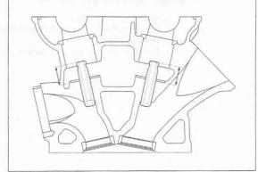
Use cutting oil on Ream the new valve guides after installation. the reamer during Insert the reamer from the combustion chamber this operation. side of the head and also always rotate the reamer clockwise.
