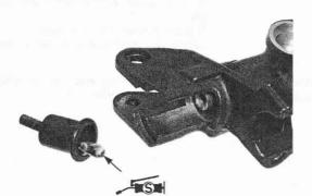
Install the clutch switch and tighten the screw to the specified torque.
