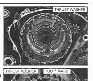
Install the clutch center and thrust washer. Install the lock washer with its "OUT" mark facing out.
