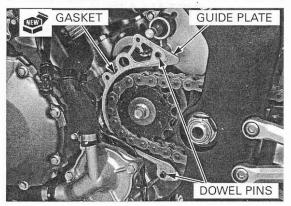
Install the left crankcase rear cover and tighten the mounting bolts.
