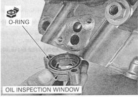
Install and tighten the bolts securely.
