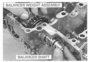
Turn the balancer shaft and place the punch mark on the shaft facing down.
