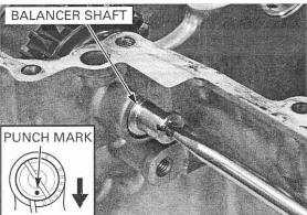
Install the balancer shaft holder.
