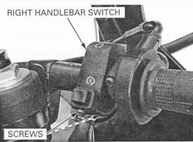
Remove the screws and throttle cable housing cover.
