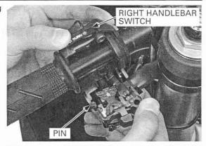
Tighten the forward screw first, then the rear screw. SWITCH HOUSING
