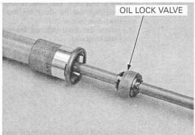
Check the fork tube for score marks, scratches, or excessive or abnormal wear.
