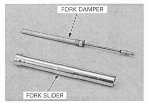
Check the oil lock valve for wear or damage. Replace the fork damper assembly, if any components are damaged.
