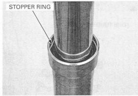
Install the dust seal into the fork slider.
