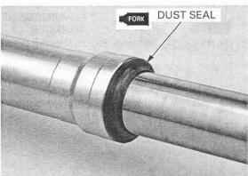
Install the fork damper assembly into the fork slider.
