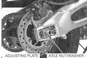
Push the rear wheel forward and derail the drive chain from the driven sprocket.
