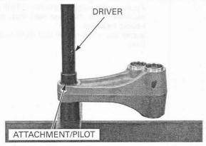
bearings into the shock arm with the. marked side facing
