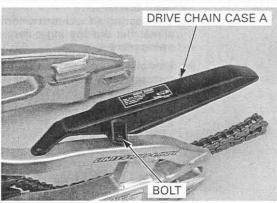
Remove the bolt, trim clip and drive chain case B.
