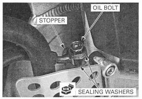
Install the reservoir and tighten the bolt to the specified torque.
