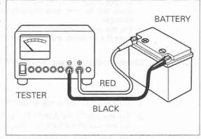
tester's cables and clamps are in good working condition and that a secure connection can be made at the battery.
