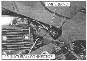
Check the resistance between three Yellow terminals of the alternator side connector.
