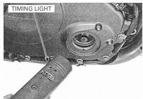
The ignition timing is correct if the "F" mark on the CKP sensor rotor aligns with the index mark on the right crankcase cover at idle.
