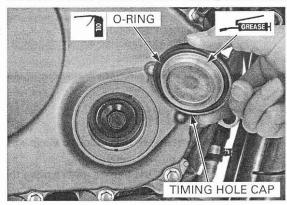
Tighten the timing hole cap to the specified torque.
