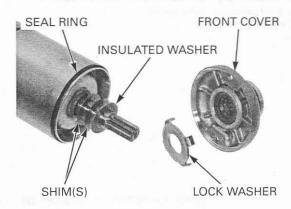
Record the location - Rear cover assembly and number of - Seal ring
