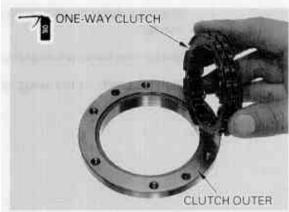
Install the starter one-way clutch assembly onto the flywheel.
