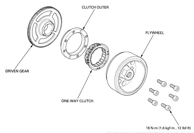
Apply oil to the starter one-way clutch. Install the one-way clutch into the clutch outer with the flange side facing in.
