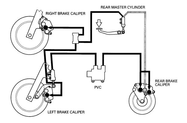
When using a brake bleeder, follow the manufacturer's operating instructions.  Connect a commercially available brake bleeder to the right front brake caliper center bleed valve.
