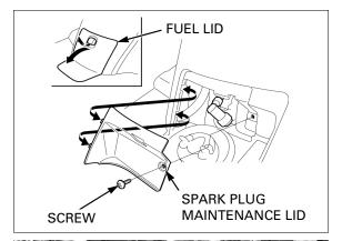
Clean around the spark plug base with compressed air before removing the plug, and be sure that no debris is allowed to enter into the combustion chamber.
