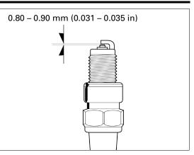
Install the spark plug in to the cylinder head and hand tighten, then tighten it to the specified torque.
