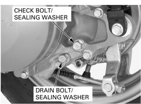
After draining the oil completely, install the drain bolt with a new sealing washer and tighten it to the specified torque.
