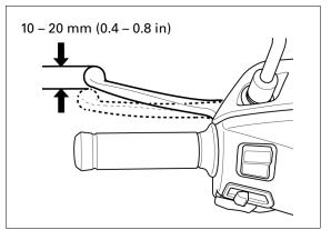
Adjust the rear brake lever freeplay by turning the rear brake arm adjusting nut.
