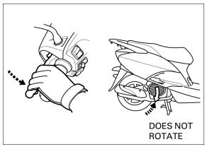
Lift the front wheel off the ground and rotate it by hand.
