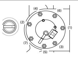
Connect the fuel pump 5P connector.
