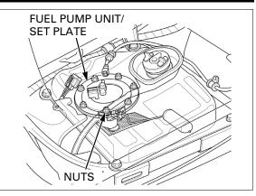
Tighten the fuel pump mounting nuts in the sequence shown.
