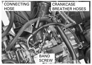
Disconnect the final reduction case breather hose from the air cleaner housing.
