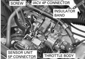
Align the throttle body tab and intake pipe tab with insulator band grooves.
