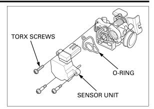
Blow open each air passage in the throttle body with the compressed air.
