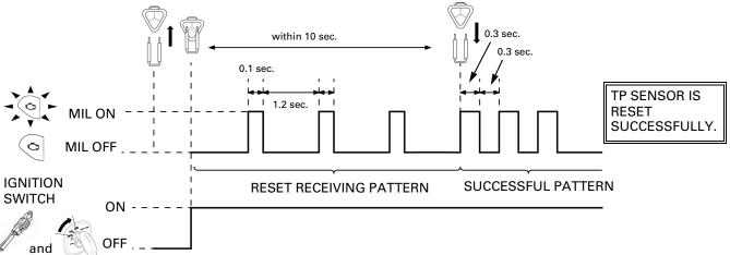
If the jumper wire is connected for more than 10 seconds, the MIL will stay ON (unsuccessful pattern). Try again from the step 4.
