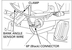
Remove the two screws and bank angle sensor.
