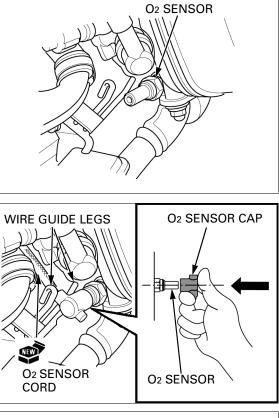
Connect the  $O_2$  sensor 2P connector.
