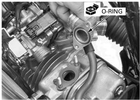
Install the insulator band to the intake pipe. Install the insulator band/intake pipe.
