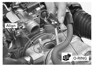
Install a new O-ring to the groove on the intake pipe.
