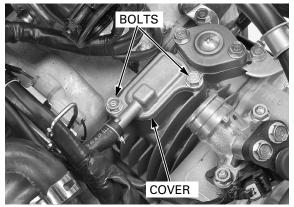
Remove the check valve from the cylinder.
