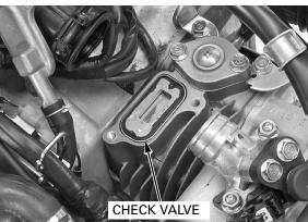
Check the reed for damage or fatigue. Replace if necessary.
