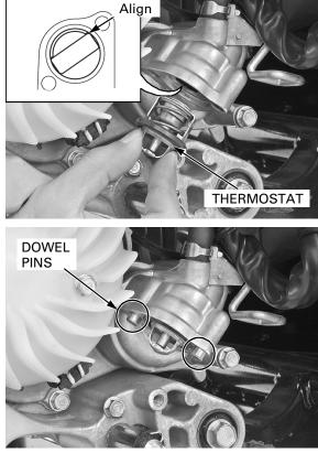
Install the dowel pins.
