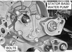
Remove the O-ring from the stator base/water pump.
