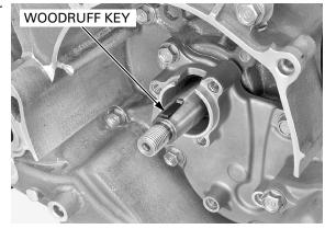
Remove the bolts and the stator base/water pump.
