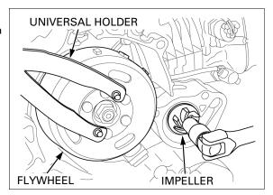
Remove the water pump impeller.
