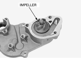
Be sure to use the hydraulic press. Do not use a hammer. Be careful not to damage the stator base/water pump mating surface.
