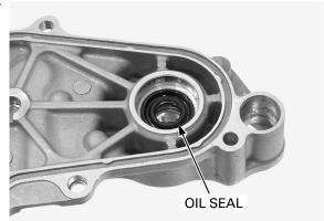
Be careful not to damage the water pump/stator base mating surface.
