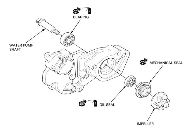
Apply engine oil to a new water pump oil seal lips.
