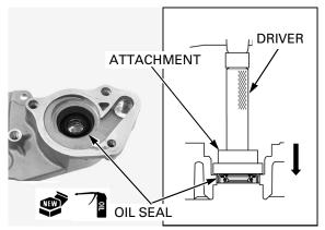
Drive a new mechanical seal until it is fully seated on the water pump groove using the special tools and hydraulic press.
