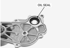
Apply engine oil to a new crankshaft oil seal lips.
