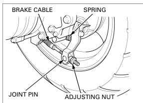
Release the rear brake cable from the cable holder and cable clamps.
