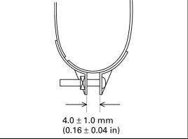
Slightly lift the rear wheel to align the bolt holes and tighten the rear shock absorber lower mounting bolt.
