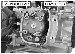
Remove the dowel pins and gasket.
