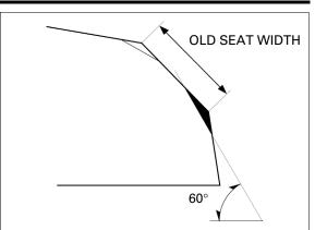
Using a  $45^\circ$  seat cutter, cut the seat to the proper width.
