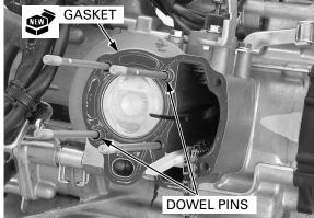
Route the cam chain through the cylinder head and install the cylinder head onto the cylinder.
