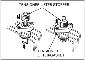
Remove the two bolts, cam chain tensioner lifter and the gasket.
