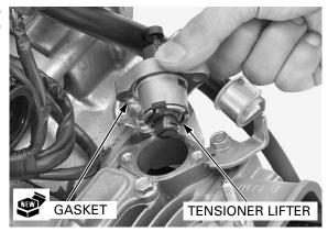
Install and tighten the bolts. Remove the tensioner lifter stopper.
