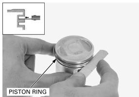
Insert each piston ring into the bottom of the cylinder squarely using the piston. Measure the ring end gap.
